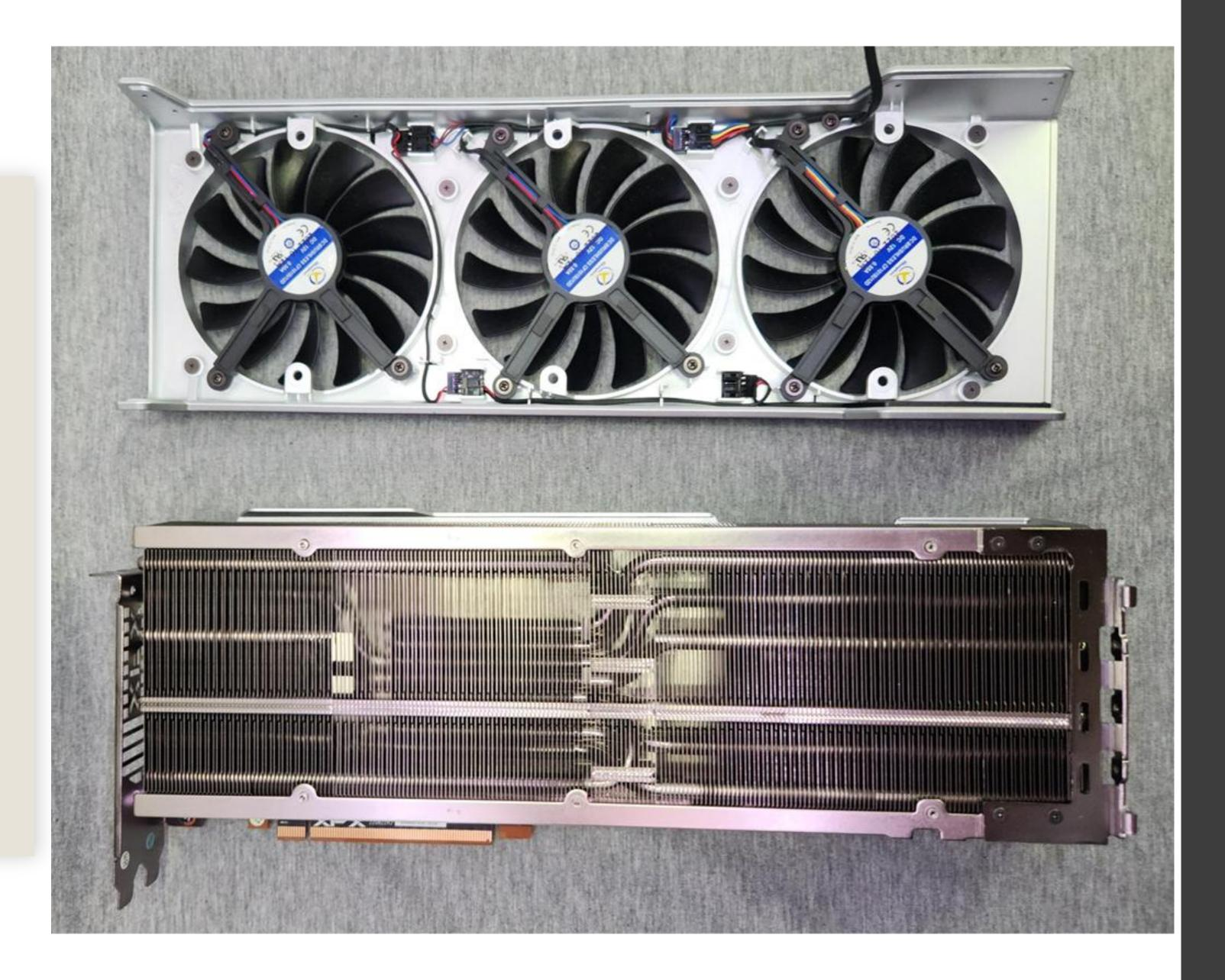
Main heatsink assembly can be removed by unscrewing all screws visible from the backplate.
