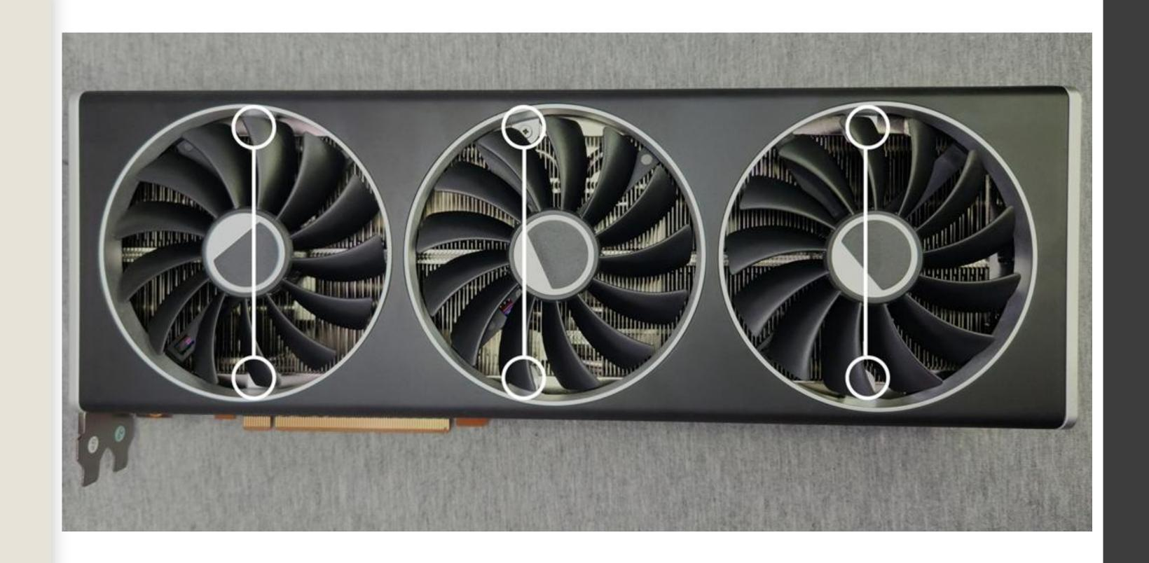
Fanshroud removed from Heatsink assembly.
