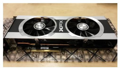
The first step is removing the faulty. If it is the front fan (nearest the DVI Ports), the removal and installation is a bit easier. If it is the back fan, or both, the removal takes 2 extra steps.
