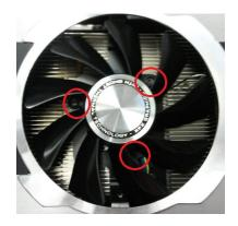
Then, take a sharp razor blade, and gently cut a slice through the protective sleeve on the fan connectors.
