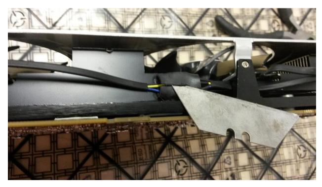
Then delicately separate the clips. Be careful not to pull the wires on this step, this particular plastic union is less durable than the clip in the PCB of the video card and can be damaged easily. It's okay to slowly jostle them free, however, some clips are very tight and require tools (like a razor blade or needle nose pliers).
