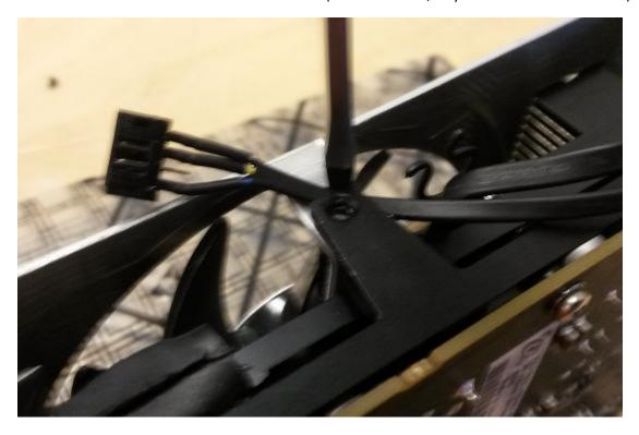
Once both screws are removed, the aluminum shroud will willingly bend inwards. Be sure to apply pressure to the Silver shroud mount, NOT the black mount. We are trying to create a gap here so the cable can be pulled through.
