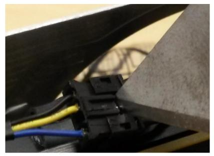
Once that is complete, you can undo the horseshoe clip by simply squeezing and separating it, or unscrewing it if you prefer. That will release the fan cable and complete this repair.
