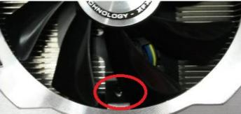
In order to remove the cables from the card, you have to remove two screws on the rear fan. The side screw (pictures above left) and the mount screw (above right) which are nearly an inch apart. Removal of these screws is needed to bend the metal inwards (toward the fan, so you can slide the cable out).
