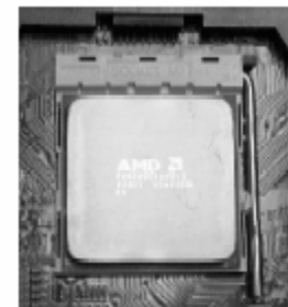
Push down the socket lever to secure the CPU
