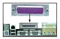
CN5 (LPT) **Connector:** 25 pin female. Type: This parallel port is used by printers which support the SPP, EPP and ECP modes IRQ7 or IRQ5 can be selected. The ECP mode will use either DMA 3 or DMA 1 (which can be selected by the BIOS setup program).
