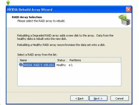
5. Select the disk in the array that was replaced and needs to be rebuilt.
