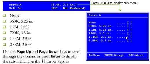
position the selector in the option you choose. Press **Enter** to accept the changes and return to the Standard CMOS Features menu.
