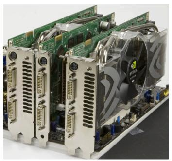
Three PCI Express graphics cards installed. Only the two outer cards will be SLI'ed using the SLI Connector
