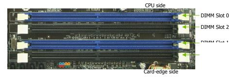
Use the following procedure to install memory DIMMs into the slots on the motherboard. Note that there is only one gap near the center of the DIMM slot. This slot matches the slot on the memory DIMM to ensure the component is installed properly.
