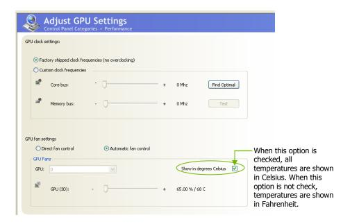
Figure 20. Adjust GPU Settings (nTune)
