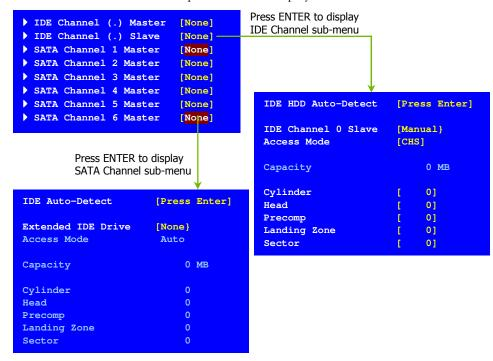
Press **Enter** to auto-detect IDE and SATA channels in the system. Once the channel is detected, the values for Capacity, Cylinder, Heads, Precomp, Landing Zone, and Sector are automatically filled in.
