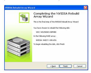
7. Click **Finish** to begin the rebuild of the selected disk in the array. (Remember that rebuilding a disk can take up to a full day.)
