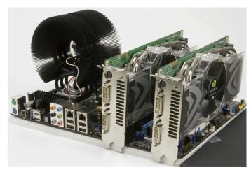
Two SLI graphics cards installed in the outer two (block) PCI Express slots on the motherboard.
